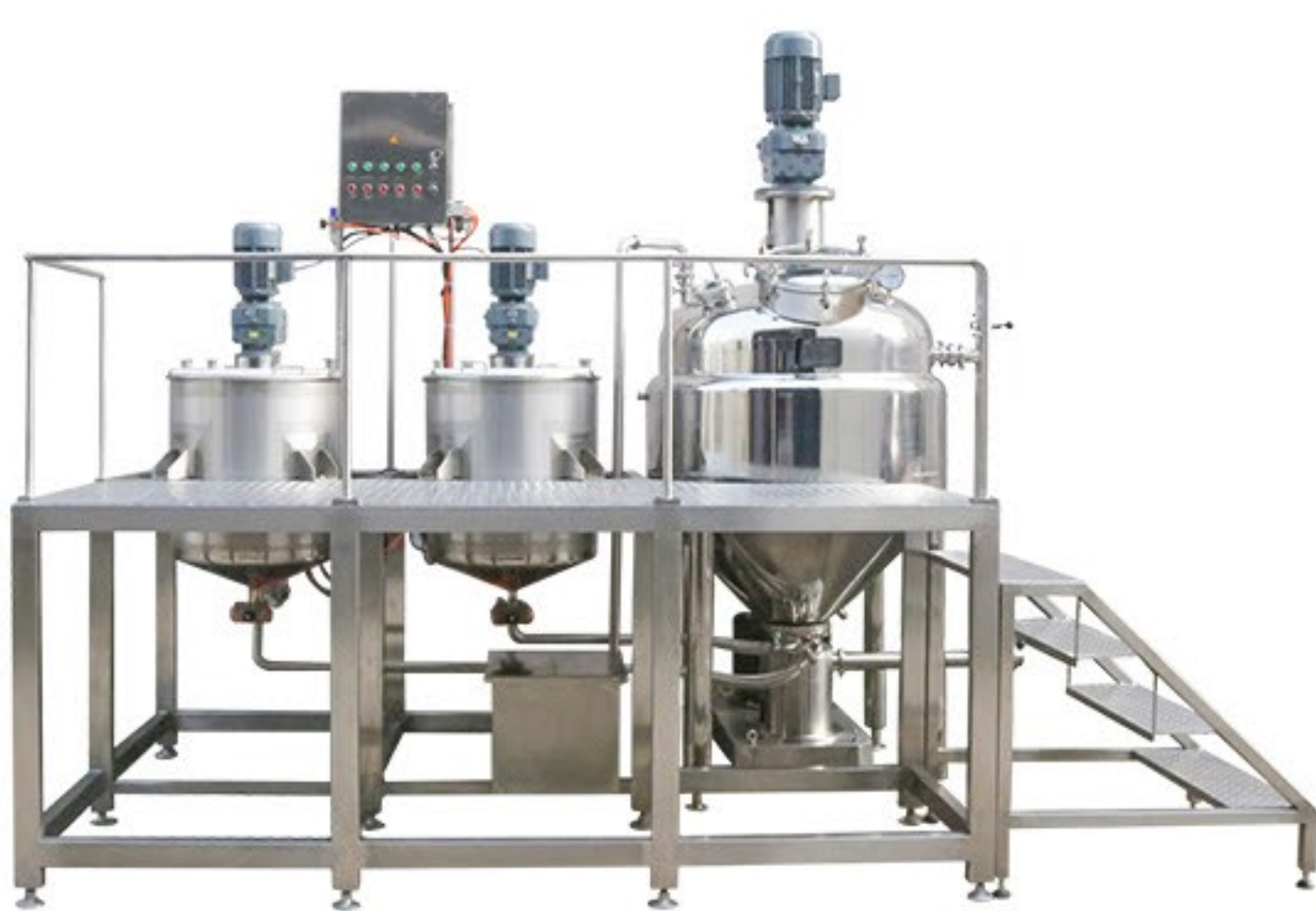
Vacuum Stirring and Emulsification System(for salad dressing)
